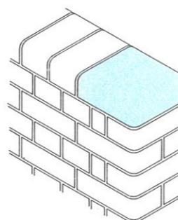
**BN.19**External return to double bullnose on edge and to bullnose double header on flat
