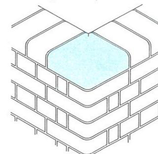
**BN.21**Double bullnose external return to double bullnose on edge and to
