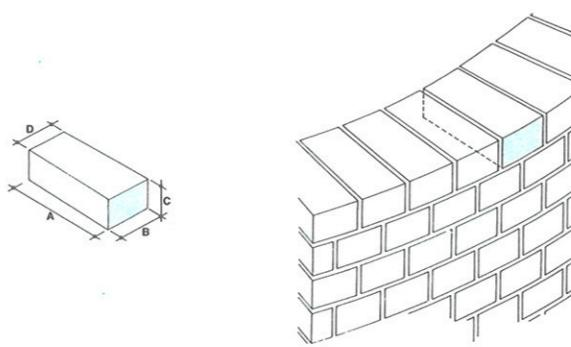
\*Dimensions B and D in types RD.1 are segmental lengths.
