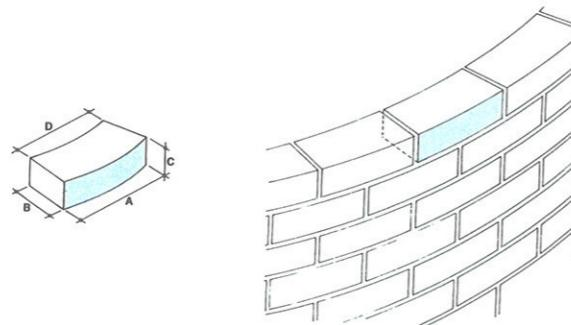
\*Dimensions A and D in types RD.2 are segmental lengths.
