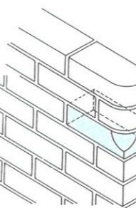
**BN.18**Stop end to double bullnose on edge and to bullnose double header on flat
